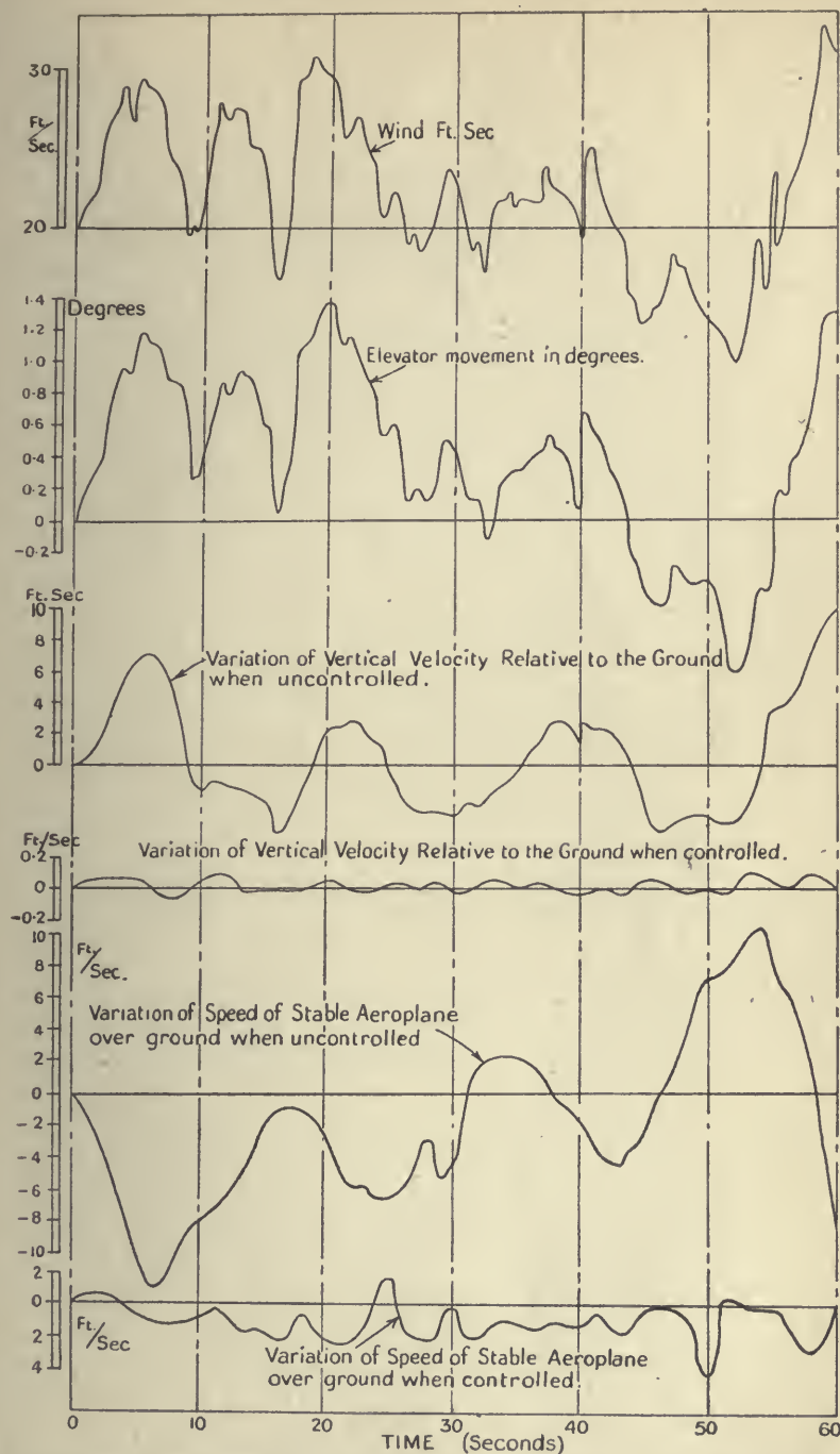
FIG. 255.—Controlled flight in a natural wind (aeroplane stable) compared with uncontrolled flight of same aeroplane.
