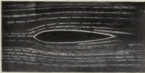
FIG. 172.—Viscous flow round strut section (free fluid).
