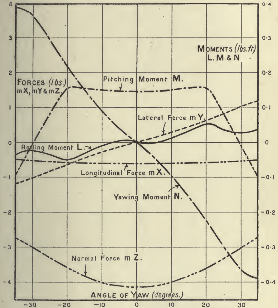
FIG. 118.—Forces and moments on complete model aeroplane referred to body axes.
