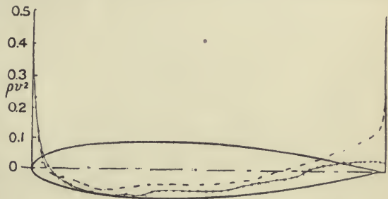
FIG. 184.—Comparison of calculated and observed pressure on a model of an airship envelope.
