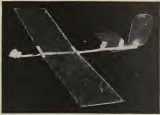
FIG. 231.—Stable model with two real fins. The dihedral fin is not actually present, but an equivalent effect is produced by the dihedral angle between the wings.
