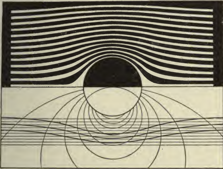
FIG. 181.—Calculated flow round circular disc for comparison with Fig. 166.
