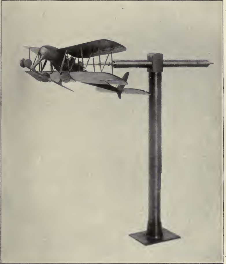
FIG. 136.—Model aeroplane arranged to show autorotation.
