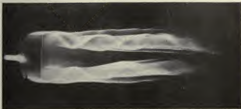
FIG. 196.—Flow of air past an inclined plate. Low speed.
