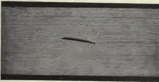
FIG. 178.—Viscous flow round wing section (Hele-Shaw).
