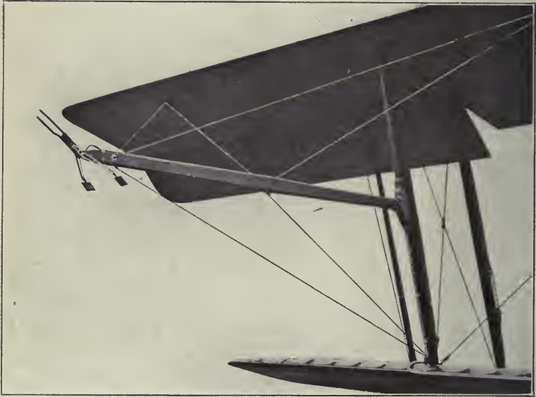
FIG. 42.—Experimental arrangement of tube anemometer on an aeroplane.
