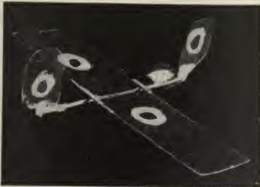
FIG. 233.—Model which illustrates lateral instabilities. (1) With front fin removed: spiral instability. (2) As shown: unstable lateral oscillation. (3) With rear fin removed: spin instability.
