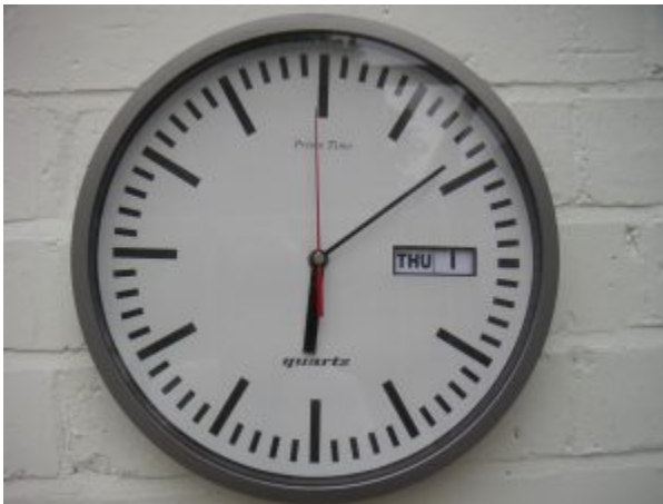
Typical wall clock with hour, minute, second hands and 1 hour, 1 min (1s) divisions. Image Credit: Clock by Lee Haywood via Wikimedia Commons
