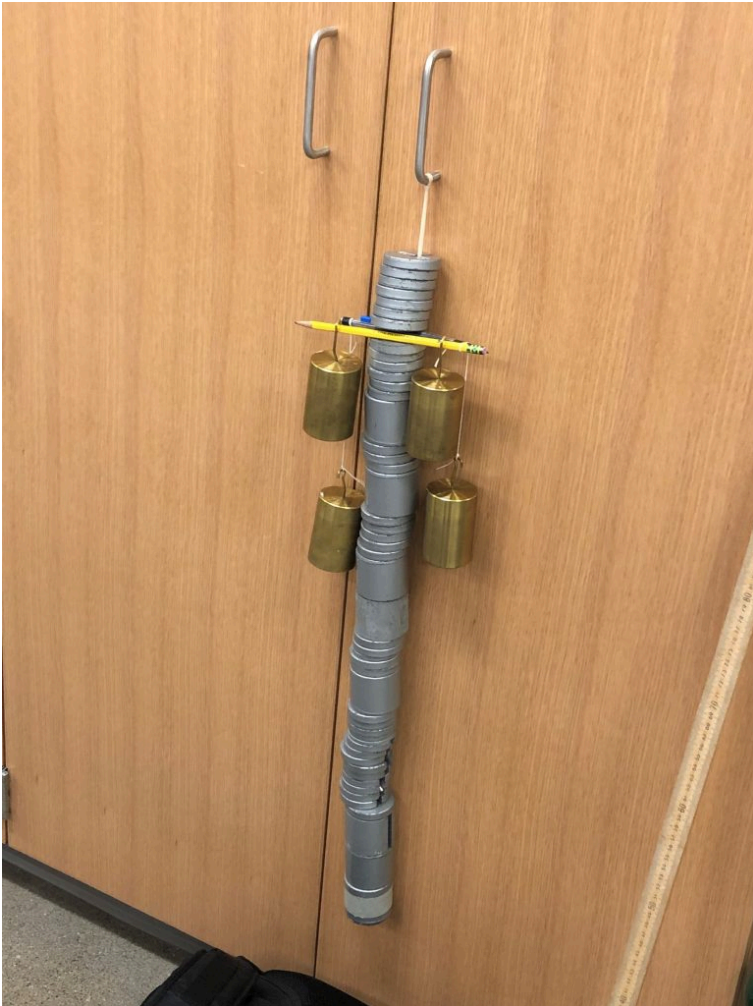
Photograph of a 1 mm x 3 mm rubber band during stress testing. The band runs through the slots in the gray weights and the hook attached to the bottom of the band is just visible through the slot in the lowest group of smaller (0.98 N) weights. The 119 N of force is applying 1.3 \times 10^{13} Pa of stress, causing a strain of 660 %. Photo credit: Umpqua Community College student Samuel Marsters.
