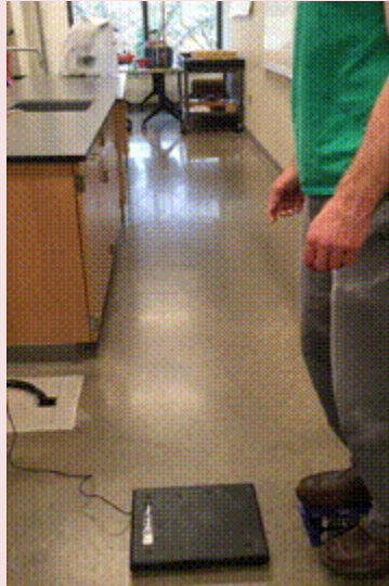
Stiff and bent-leg landings that produced the force vs. time data shown below.
