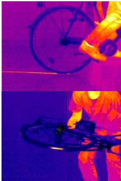
k / An infrared camera distinguishes hot and cold areas. As the bike skids to a stop with its brakes locked, the kinetic energy of the bike and rider is converted into heat in both the floor (top) and the tire (bottom).
