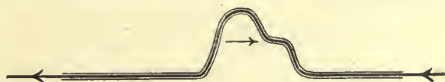
FIG. 131. — Illustrating how centrifugal force balances stretching force when a transverse wave traverses a string.
