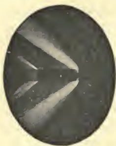
FIG. 140.—Showing the compressions and rarefactions which accompany a rifle ball in its flight.
