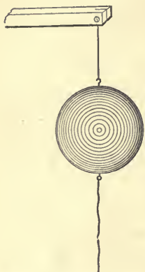
FIG. 41. — Illustrating reaction which is measured by mass \times acceleration.
