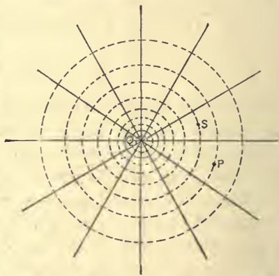
FIG. 250. — Illustrating the relation between lines of force and equipotential surfaces.
