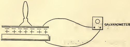
FIG. 258. — Showing the current which is produced when an electrophorus is discharged.
