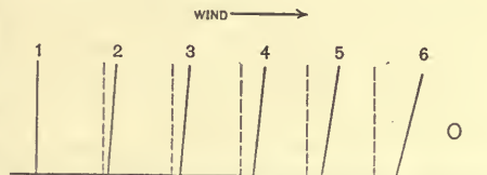
FIG. 157.—Sound traveling with wind. Dotted lines show successive positions of wave front in still air.
