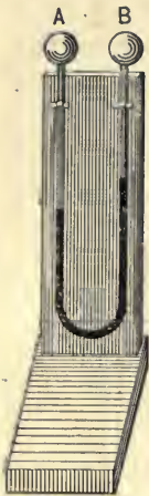
FIG. 175. — Schoot's differential thermometer.
