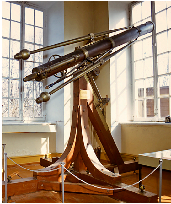
Figure 7: Wilhelm Struve’s 24-cm refractor, Tartu. This was used in the 1830s to measure one of the first stellar parallaxes, that of the bright star Vega (courtesy Tartu Observatory, Estonia).
