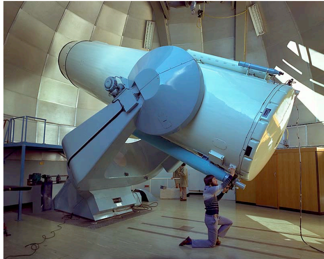
Figure 10: The UK 1.2-meter Schmidt telescope at the Anglo–Australian Observatory, Australia (1977), used for large-scale photographic surveys of the southern skies from the 1970s (courtesy Australian Astronomical Observatory and David Malin Images).
