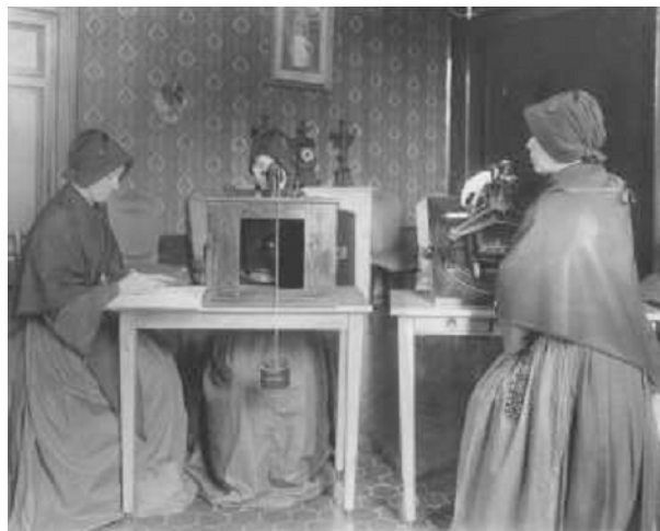
Figure 12: Nuns measuring the Vatican Zone Carte du Ciel plates, c1900 (courtesy Torino Observatory).
