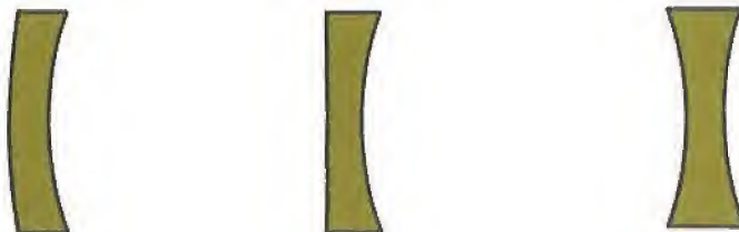
Fig. 11-3 Meniscus, Plano-Concave, and Double-Concave Diverging Lenses
