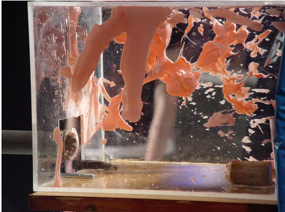
Figure 3: Collision event of the vacuum cannon as displayed in our plastic detector. The wooden projectile can be seen on the lower right.
