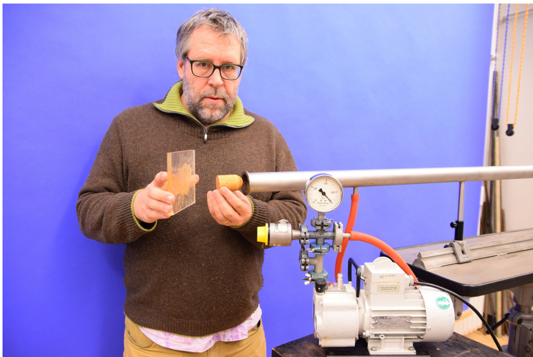
Figure 55: One of us (HKD) with the injection side of the vacuum cannon. The vacuum pump as well as the hook-up via the red rubber hose is shown. The wooden projectile is just at the entrance to the pipe, together with the greased plastic plate seal.
