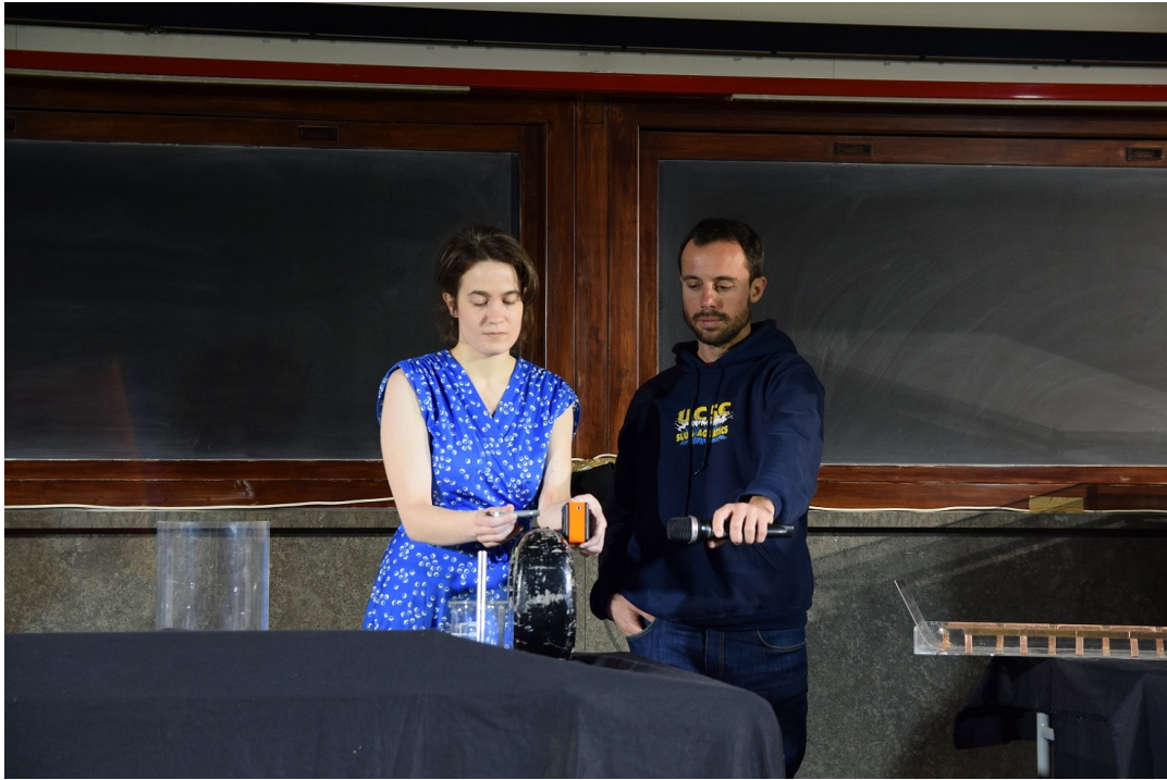
Figure 10: The beta-decay matter and anti-matter experiment, with JSch-R (Jane) and LU. The orange box is the Geiger counter. The black object underneath and slightly to the left is the magnet. One source is the silver pen in JSch-R's right hand. The other source is in the glass.
