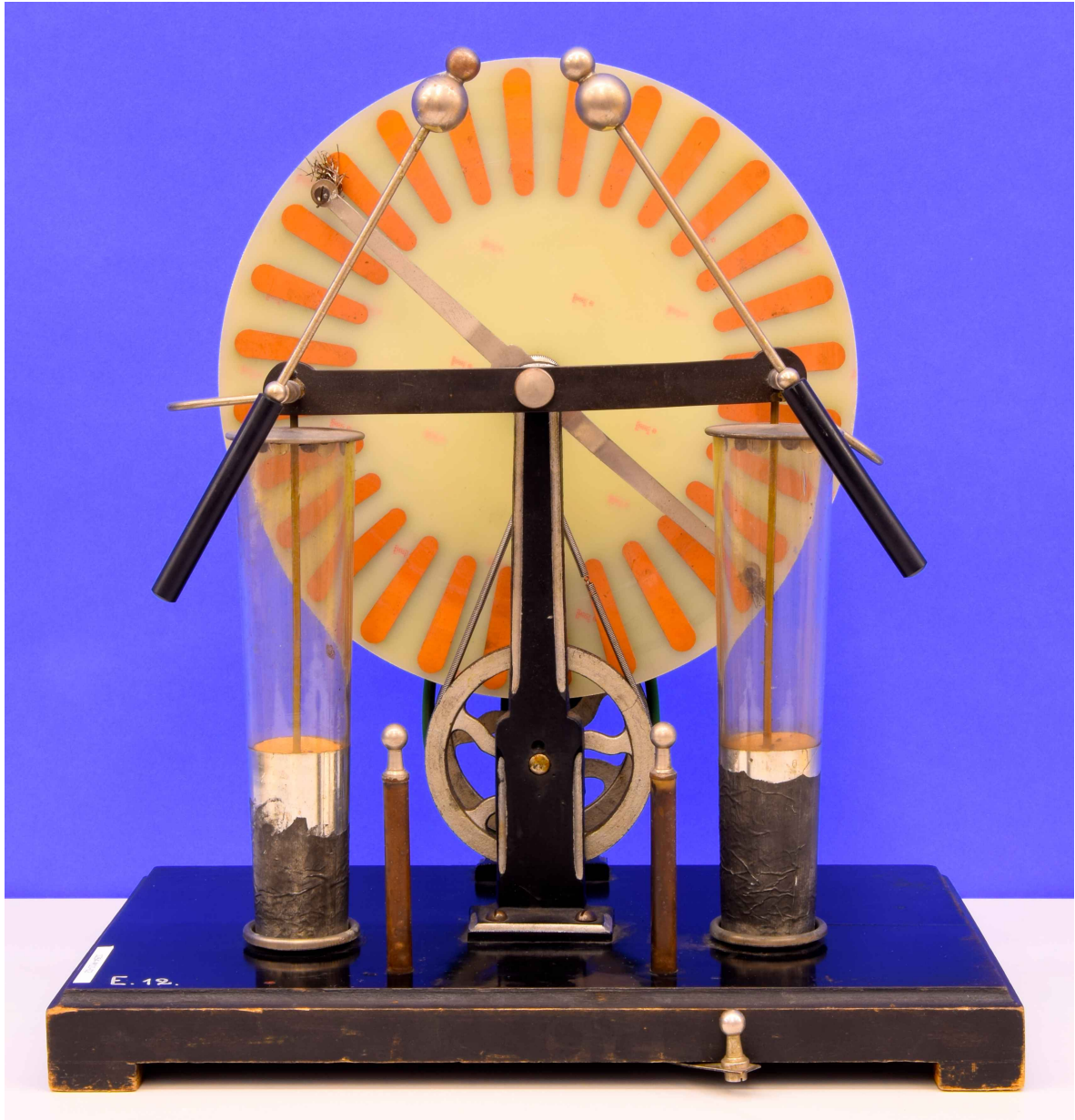
Figure 48: In the show we power the accelerator with this electrostatic generator out of our collection. It is a Wimshurst influence machine, which produces a direct current (DC). We consider it less abstract than a modern power source. The cylindrical objects on the left and right are Leyden jars, which enable more charge collection and thus higher voltages. This experiment is from around 1930. The rotating circular discs with the copper contacts have been restored.
