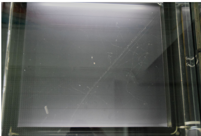
Figure 42: A top view photo of the PHYWE cloud chamber, while in operation. An unusually long track can be seen here diagonally across the chamber, most likely a muon. In the lower left corner is also a thick track from a hadron, corresponding most likely to an alpha particle.
