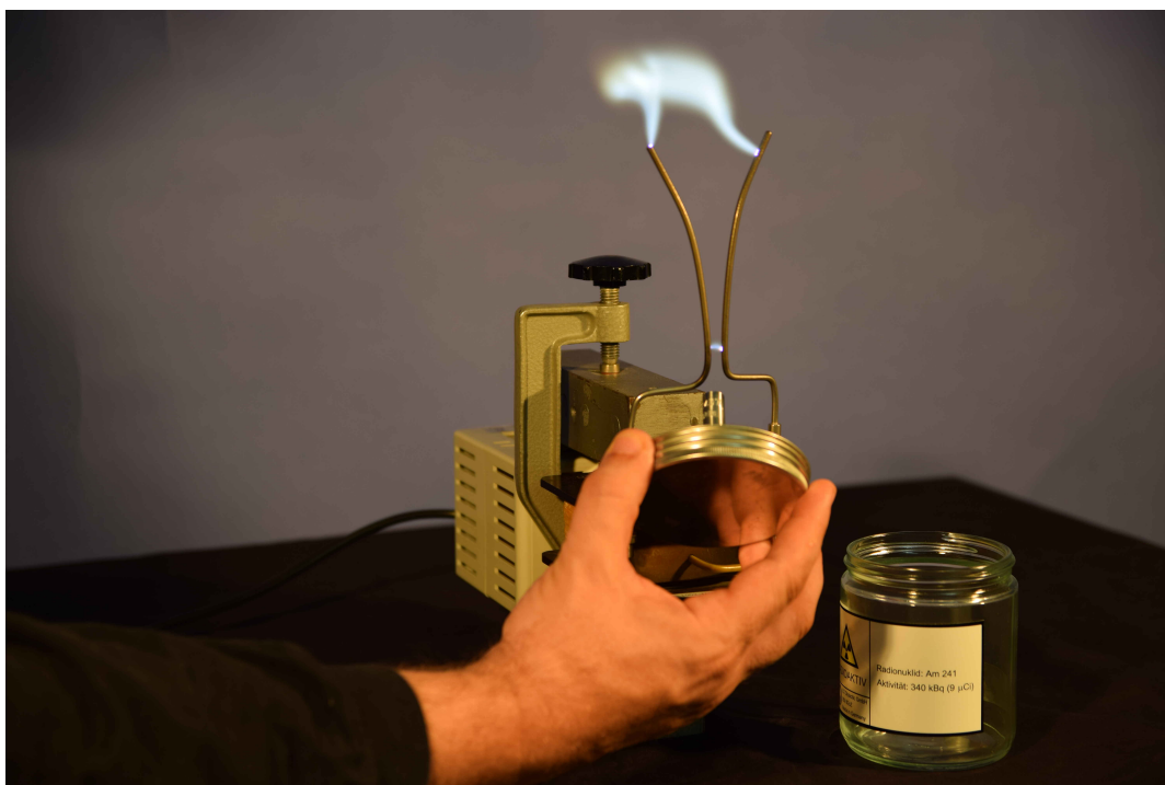
Figure 40: The Jacob's Ladder activated here by a radioactive \text{Am}^{241} source. With a radioactivity of 340 kBq the source required a 200 V potential and 5 mm of separation between the bars. We are not allowed to transport such a strong source.
