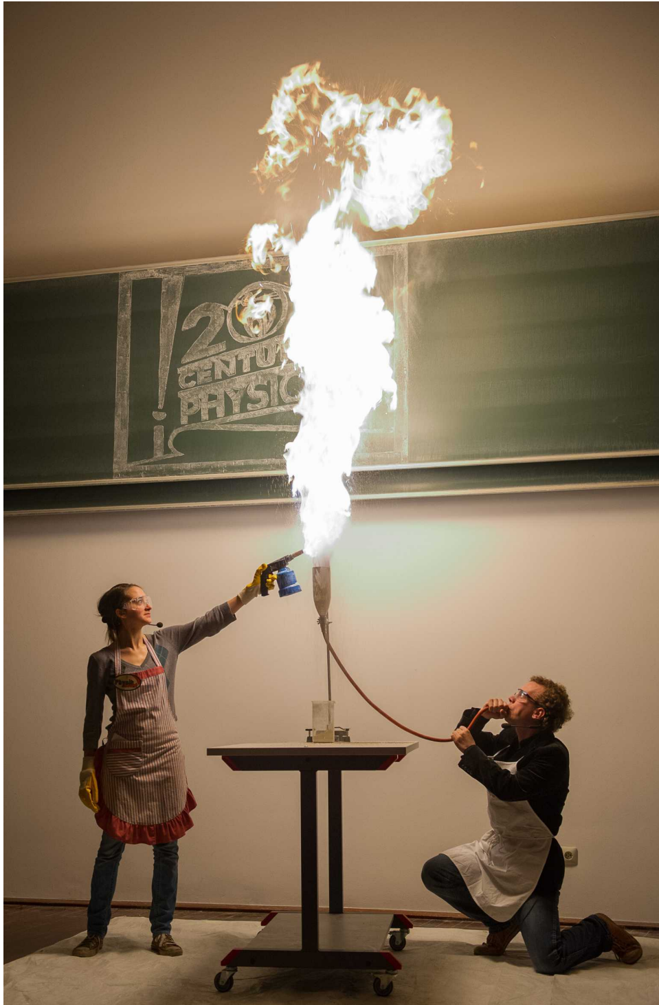
Figure 13: Burning flour cloud with Sina Kürtz on the left and DH on the right. The cut-off PET bottle is filled with flour. The latter is ejected upwards, by blowing through the red rubber hose. The floor is covered by a fire-proof tarp. This is from a different Bonn physics show. Photo by Volker Lannert.
