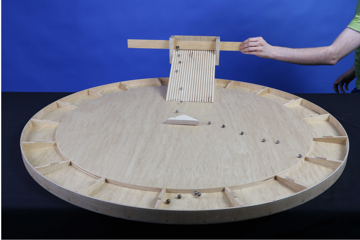
Figure 32: Wooden scattering experiment. The steel balls roll down the incline and hit the central target, here a triangular piece of wood. The target can be replaced by other shapes. The outside ring is lowered and divided into 18 equal-sized pockets, of scattering angles \Delta\phi = 20^\circ , where the steel balls are collected and counted.
