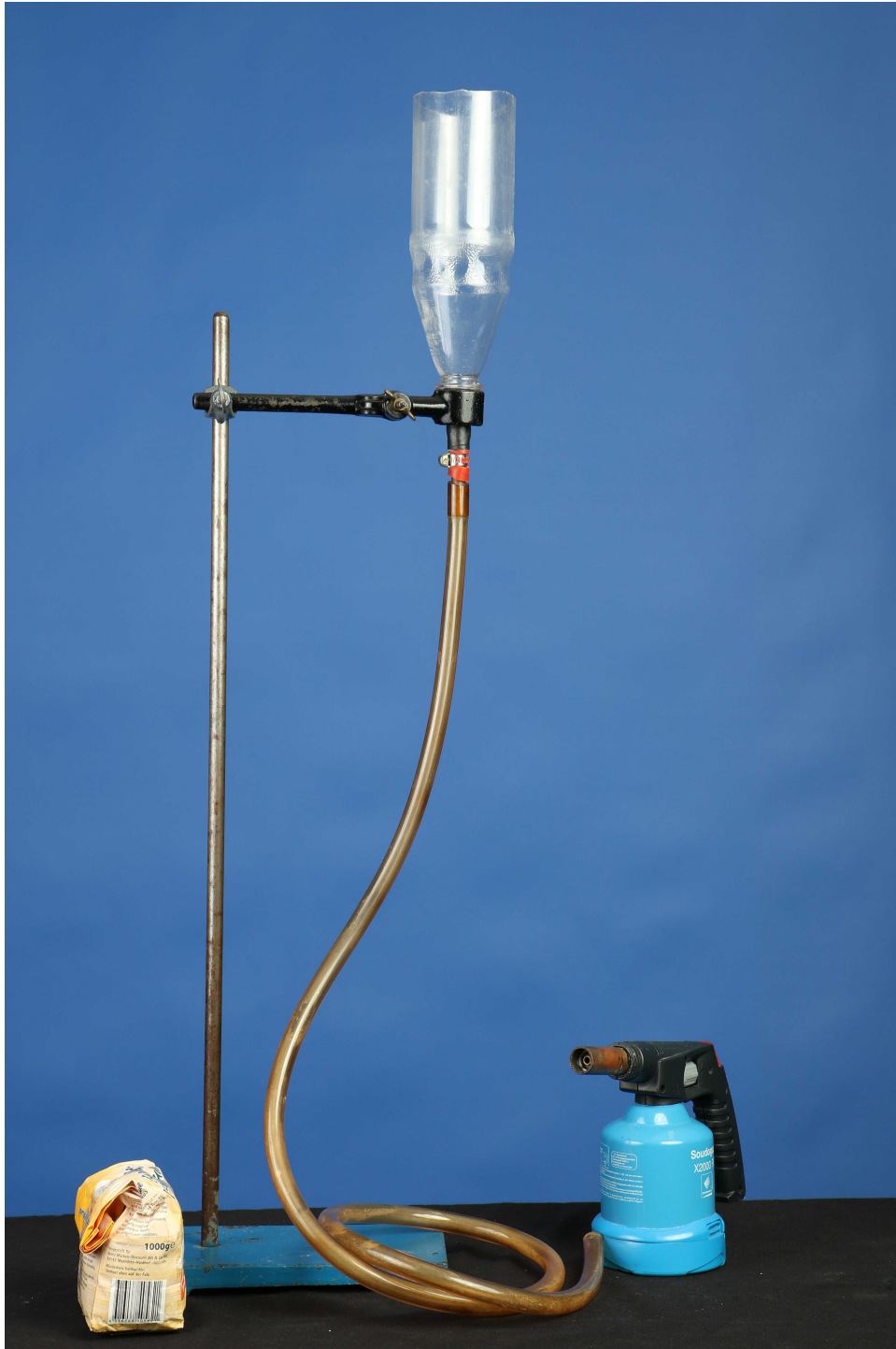
Figure 53: Close-up of our flour explosion experiment. On the left the conventional baking flour. On the right the gas blow-torch. the support structure holds the inverted and cut plastic bottle. A long tube is connected to blow into the bottom of the bottle from a safe distance.
