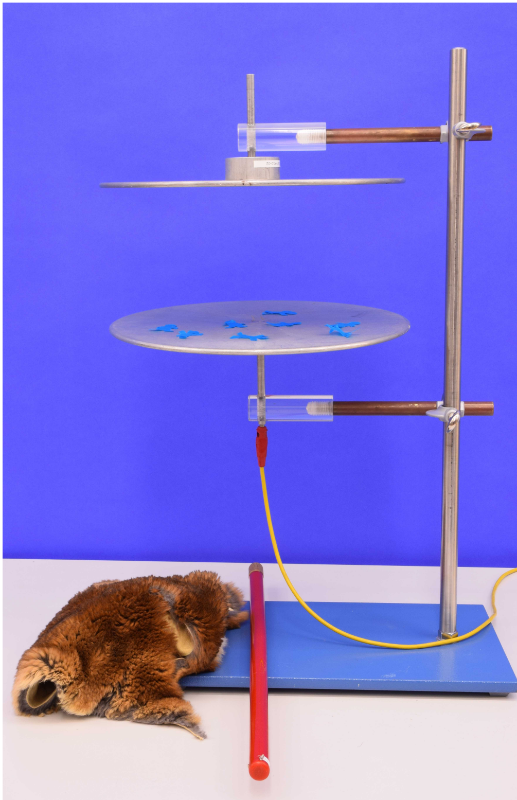
Figure 46: The complete experiment. On the left is the cat fur next to the red plastic rod. The two plates are electrically isolated from the support structure. The bottom plate is connected to Earth.
