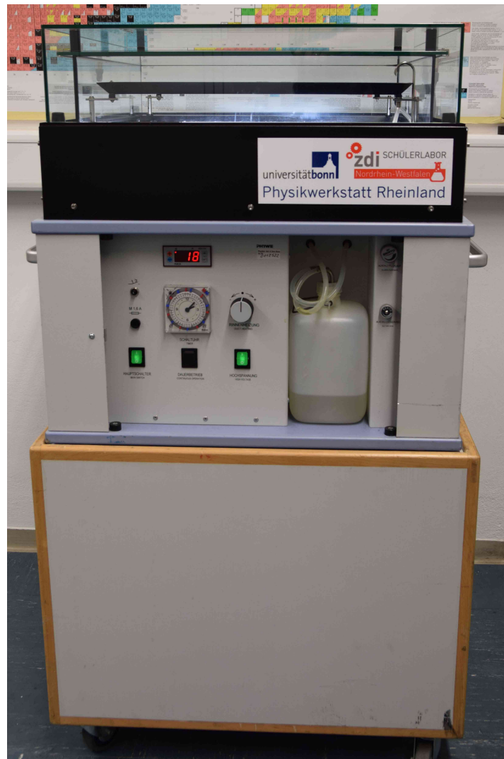
Figure 41: The PHYWE cloud chamber. The upper black part with the glass casing contains the actual chamber. Underneath is the electronics and the refrigeration unit. The plastic container on the right holds the 2-propanol. The wooden box is on wheels for easy transport. It also raises the chamber to a height easily visible for adults.
