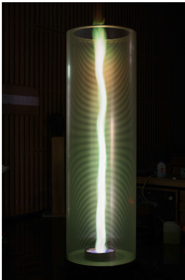
Figure 28: Fire tornado in our 2 m high rotating cage.
