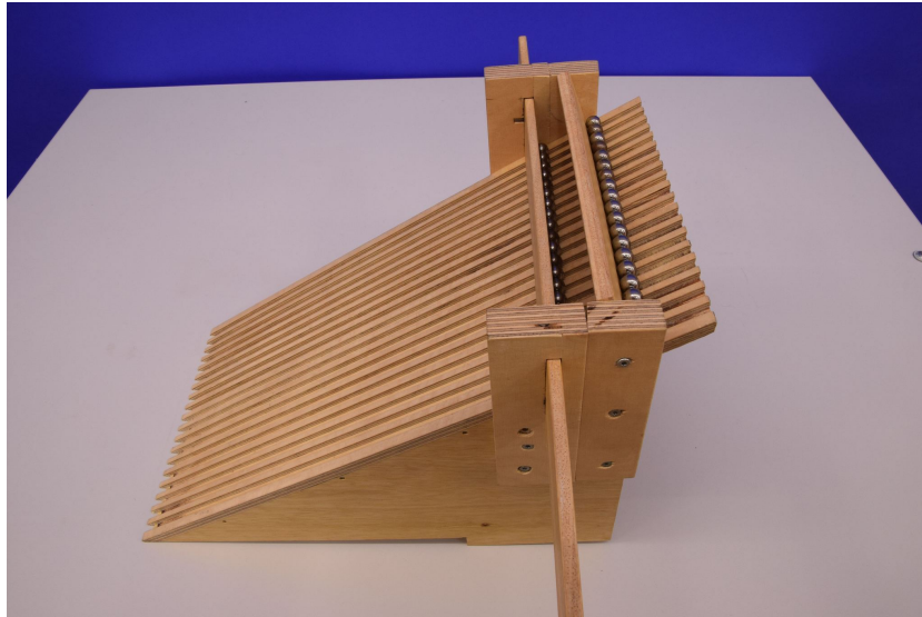
Figure 34: The reloading mechanism. The board holding the upper row of steel balls is easily rotated, releasing all balls to the lower level.
