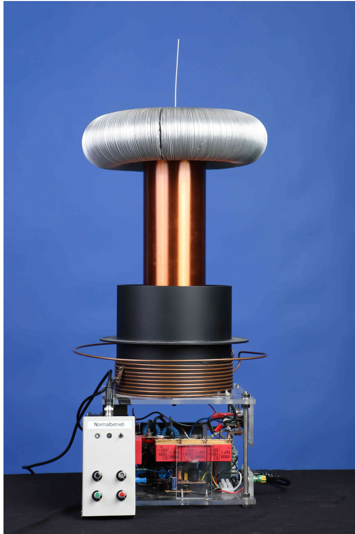
Figure 67: Our Tesla transformer, built by Timo Poller. The gray box on the left contains the remote controls connected to the transformer via an extended cable.
