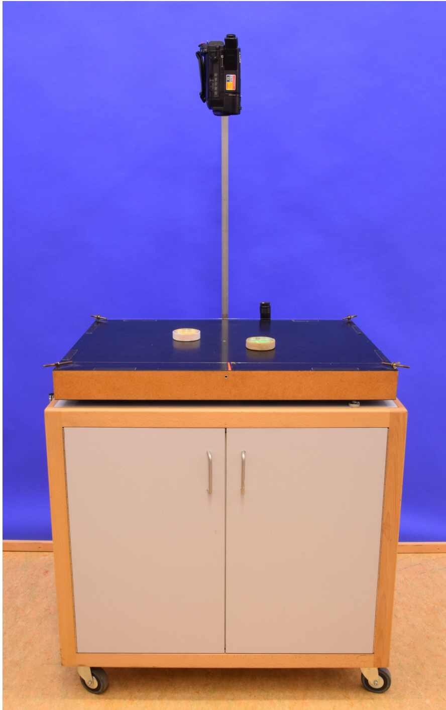
Figure 58: Overall view of the air table with two pucks on it. On top is the camera, which we use to project the puck interactions onto the big screen. The cabinet underneath contains the air pump. You can also clearly see the taut wires, which keep the pucks on the table.
