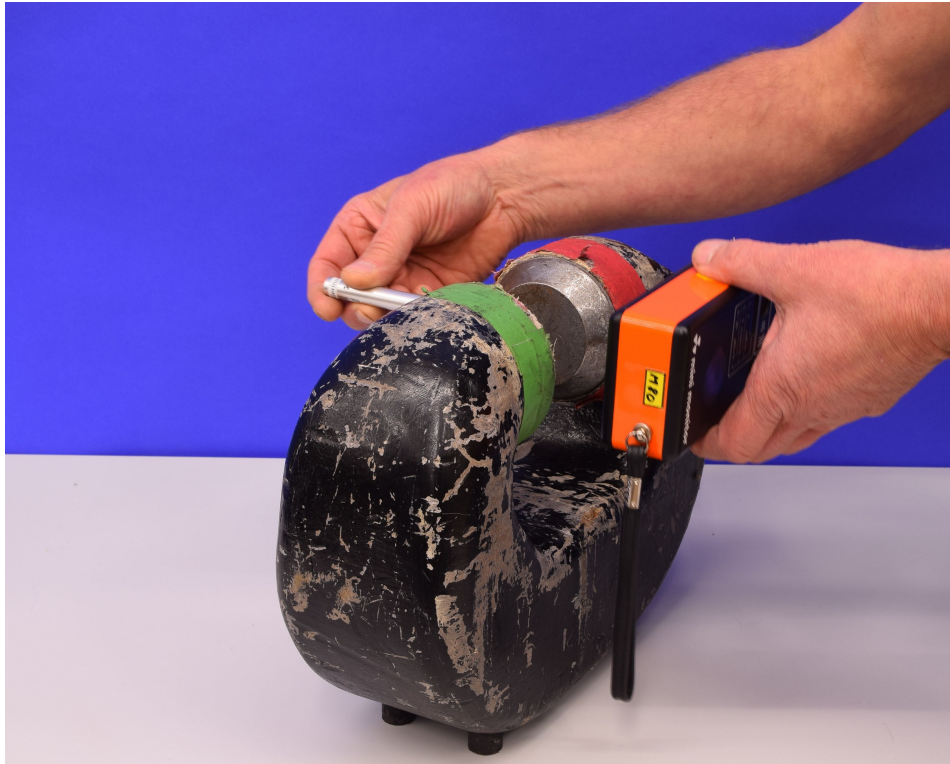
Figure 43: The horseshoe-shaped magnet. On the left, the silver, pen-like object is a beta emitter, on the right, in orange and black, is a Geiger counter.
