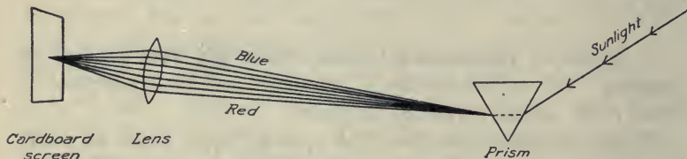
FIG. 32. — The prism refracts and disperses the light. The lens combines the color rays again, producing white light — analysis and synthesis of sunlight.
