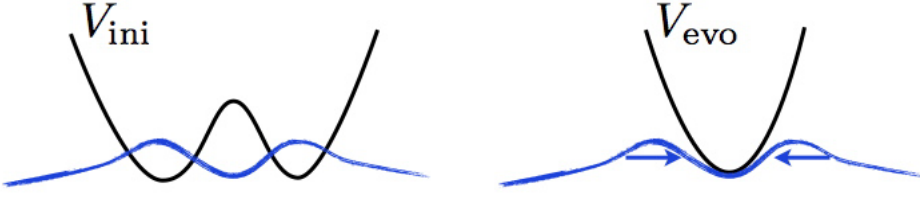
Figure 1.1: A sudden change of the shape of the longitudinal potential induces a large-scale motion in the gas.
