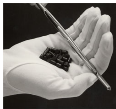
n / These pellets of uranium fuel will be inserted into the metal fuel rod and used in a nuclear reactor. The pellets emit alpha and beta radiation, which the gloves are thick enough to stop.
