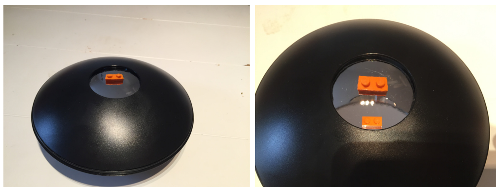
FIGURE 129 A floating Lego brick displayed by two stacked parabolic mirrors, the upper one with a hole. The right picture shows both the brick lying at the bottom and the floating image. (© Christoph Schiller).
