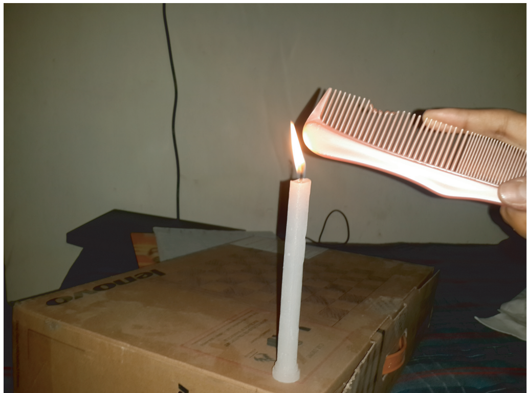
FIGURE 187 The way a flame reacts to a rubbed comb (© Shubham Das and Rakesh Kumar).
