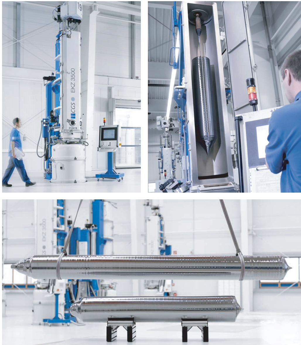
FIGURE 48 A silicon crystal growing machine and two resulting crystals, with a length of c. 2 m (© www.pvatepla.com ).
