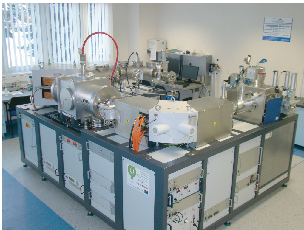
FIGURE 108 A modern accelerator mass spectrometer for radiocarbon dating, at the Hungarian Academy of Sciences (© HAS).
