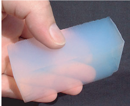
FIGURE 67 A piece of aerogel, a solid that is so porous that it is translucent (courtesy NASA).
