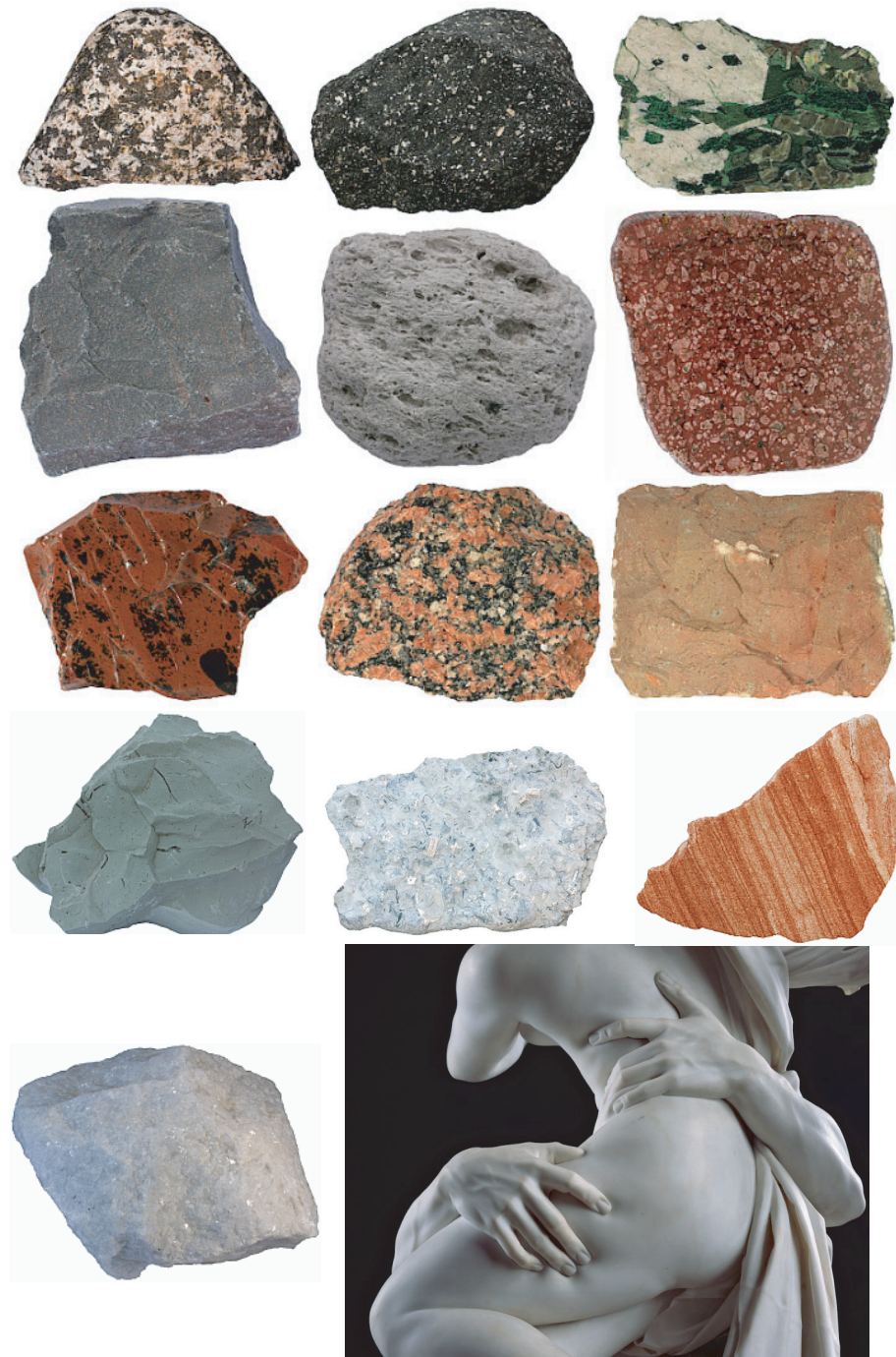
FIGURE 26 Igneous rocks (top three rows): gabbro, andesite, permatite, basalt, pumice, porphyry, obsidian, granite, tuff; sedimentary rocks (centre): clay, limestone, sandstone; and (below) two specimen of a metamorphic rock: marble (© Siim Sepp at www.sandatlas.org , Wikimedia).
