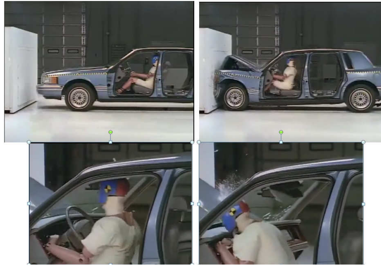
Figure 1.10 A car and its passenger are moving at the same velocity. The car suddenly decelerates. The friction force between the seat and the passenger is insufficient to significantly the velocity of the dummy.
