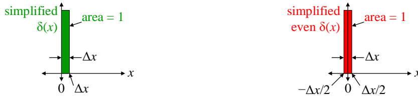
Figure 2.1 (Left) The \delta -function can be written as one-sided in most cases. However, (right) it is usually considered even. In any case, we take the limit as \Delta x \rightarrow 0 .
