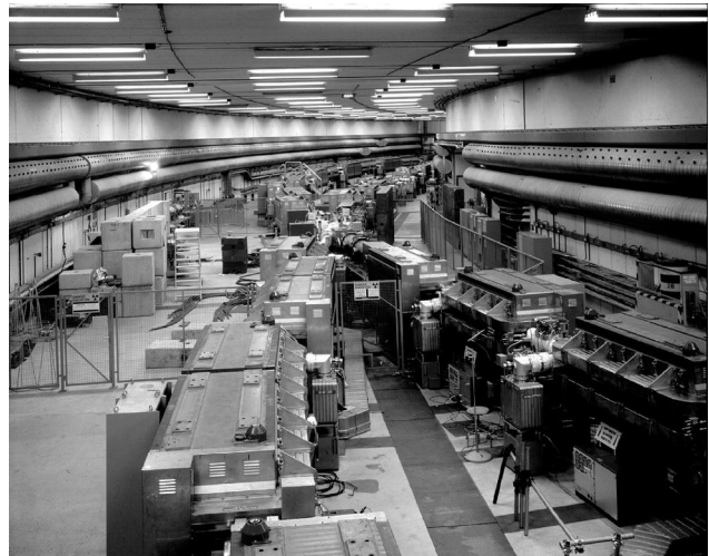
FIGURE 17 One of the intersecting points in the intersecting storage ring at CERN. The large blocks are quadrupole magnets. The intersection of the two vacuum chambers can be clearly seen. [Courtesy of CERN.]
