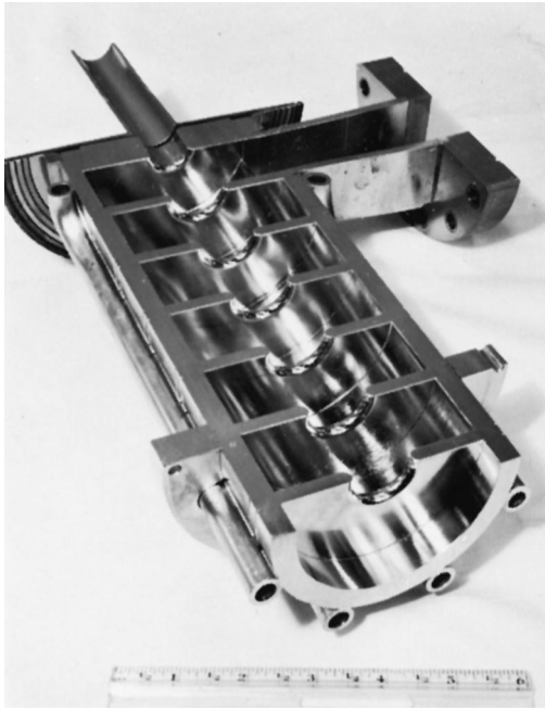
FIGURE 12 Cutaway view of a traveling-wave waveguide. The radio-frequency wavelength used is approximately 10 cm. The beam enters from the upper left and passes through the small hole. Radio-frequency power is brought in at the upper right, and the wave travels with the beam. [Courtesy of Stanford Linear Accelerator Center.]
