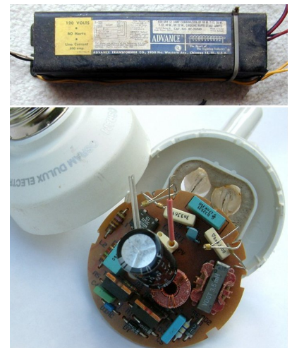
n / Ballasts for fluorescent lights. Top: a big, heavy inductor used as a ballast in an old-fashioned fluorescent bulb. Bottom: a small solid-state ballast, built into the base of a modern compact fluorescent bulb.
