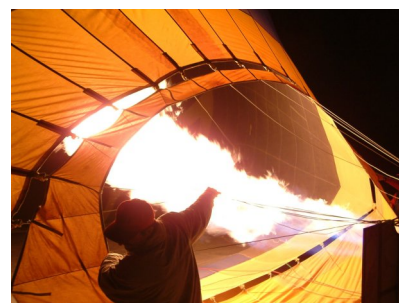
g / A hot air balloon is inflated. Because of thermal expansion, the hot air is less dense than the surrounding cold air, and therefore floats as the cold air drops underneath it and pushes it up out of the way.
