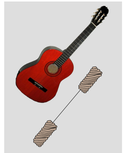
l / We model a guitar string attached to the guitar's body at both ends as a light-weight string attached to extremely heavy strings at its ends.
