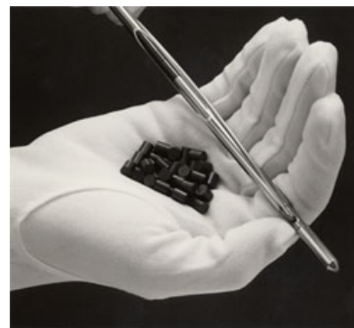
d / These pellets of uranium fuel will be inserted into the metal fuel rod and used in a nuclear reactor. The pellets emit alpha and beta radiation, which the gloves are thick enough to stop.
