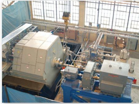
*36.5 MW HTS Ship Drive Motor
