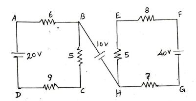
28. Using Thevenin theorem, calculate the current flowing through the load resistor  $R_L = 5\Omega$ .
