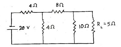
29. Calculate the value of R which will absorb maximum power from the following circuit. Also, compute the value of maximum power.
