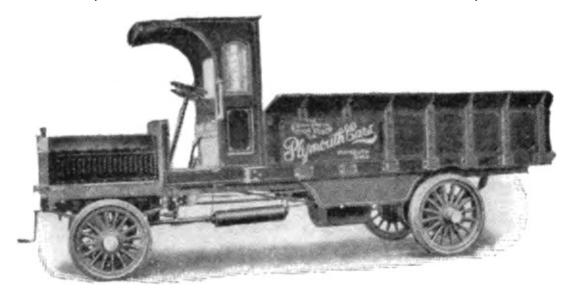
BODY: Side board truck CAPACITY: 2 to 3 tons WEIGHT: 4,500 pounds WHEEL-BASE: 144 inches
