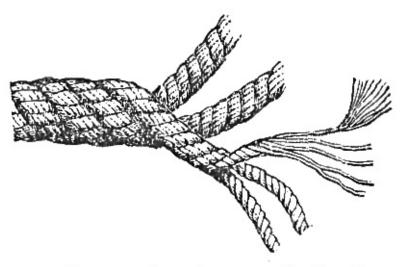
Rope, showing method of construction.
