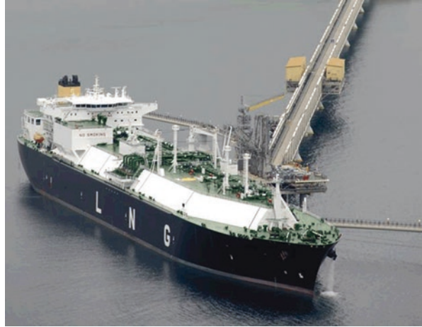
Fig. 2.1 130,000 m 3 LNG carrier with integrated Invar tank
