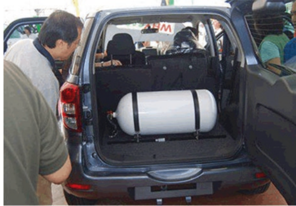
Fig. 4.12 Utilization of compressed natural gas as fuel
