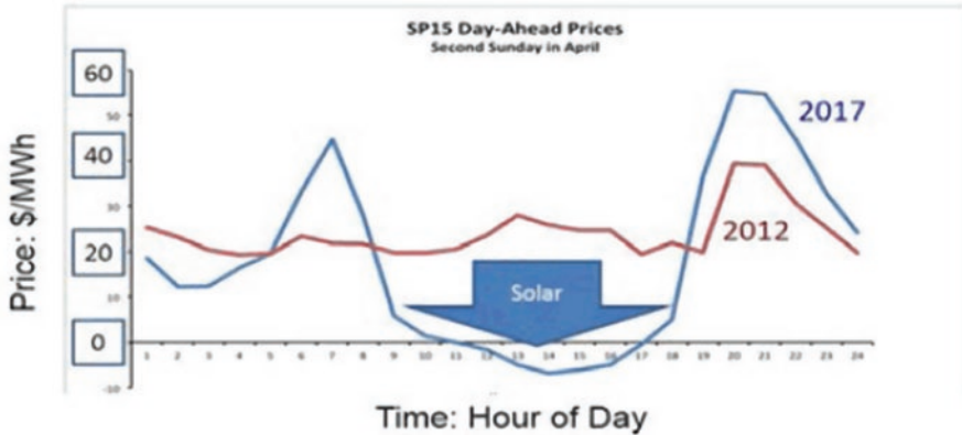
Fig. 7.1 Impact of added solar on California electricity prices for second Sunday in April 2012 and 2017
