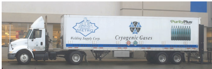
Fig. 2.24 Cryogenic gases delivery truck at a supermarket
