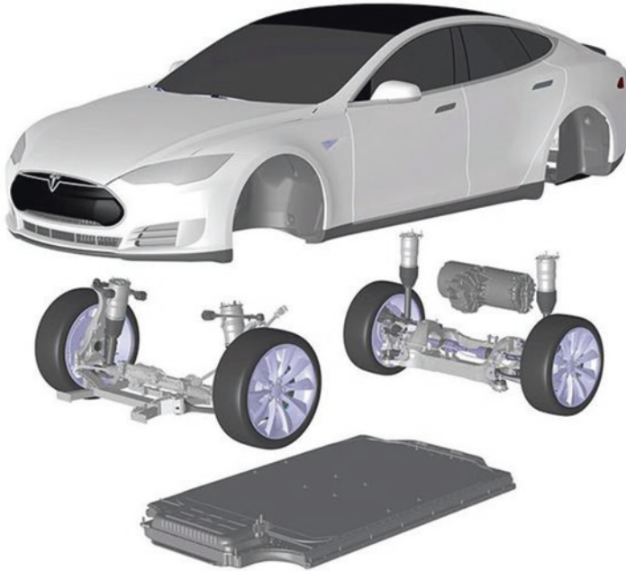
Fig. 8.26 Tesla's battery pack in the floor pan of the model S (Courtesy of Tesla Corporation)
