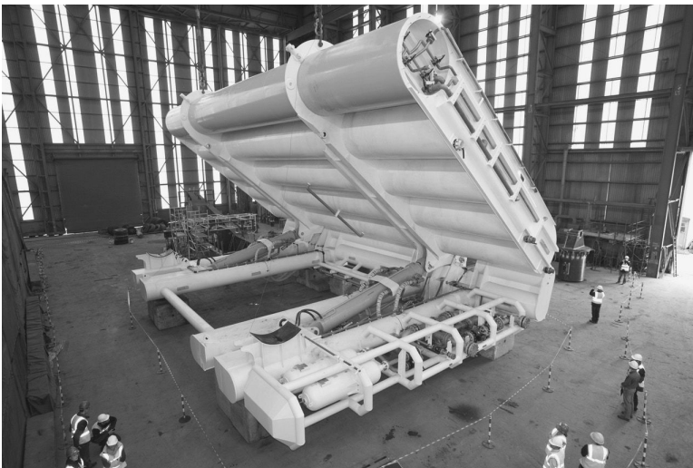
FIGURE 12.27 Oyster hydroelectric wave energy converter, 315 kW; unit installed at Billa Croo, Orkney, Scotland. (Courtesy of Aquamarine Power.)
