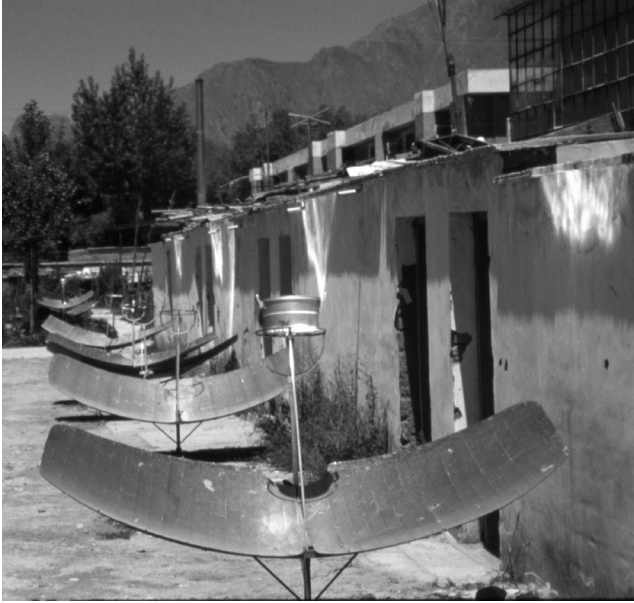
FIGURE 5.27 Each family at the Solar Energy Research Institute, Lhasa, Tibet, has a concentrating solar cooker to heat its teakettle.
