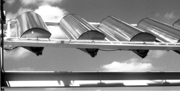
FIGURE 7.12 Linear Fresnel lens, PV strip (4 cm wide) at focus, two-axis tracking, system (around 400 W per unit), 300-kW array, at 3M Research Center in Austin, Texas (1990). Notice fins on the back for heat dissipation.
