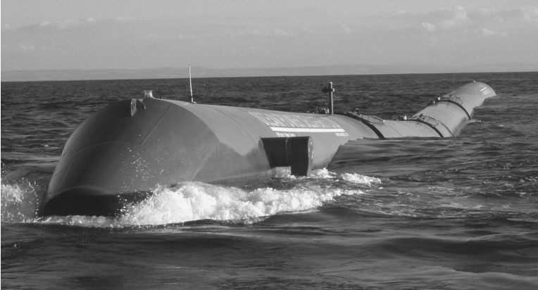
FIGURE 12.23 Sea trial of Pelamis Wave Energy Converter, 750 kW. (Courtesy of Pelamis Wave Energy.)
