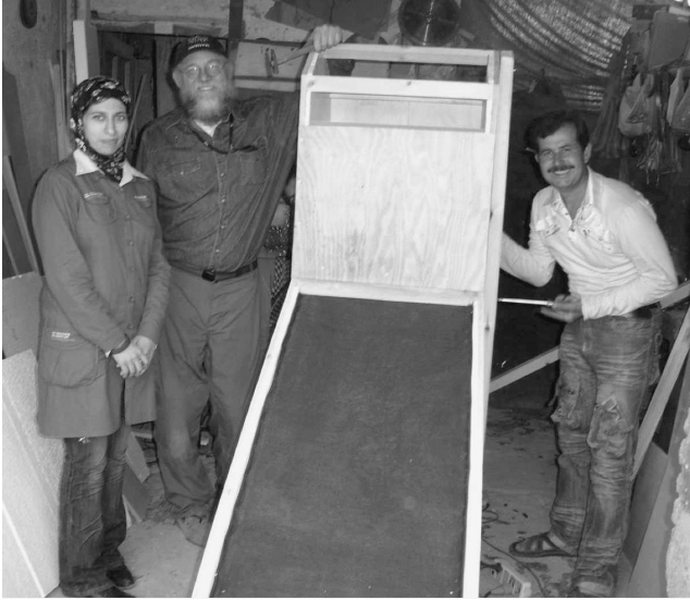
FIGURE 5.23 Indirect dryers built at local shop, Kabul, Afghanistan. In 2009, there were 130 built. Left to right: Khatera Obaid, Robert Foster, and carpenter Mohammad Hakeen Popa. (Courtesy of Mohammad Salim.)
