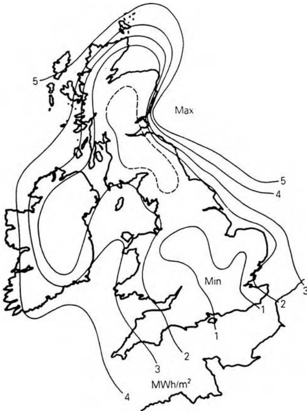
FIGURE 3.22 Wind energy map of the U.K. in MWh/m 2 per year at open sites, excluding hilltops. (From Freris, L.L., Wind Energy Conversion Systems , Prentice Hall, London, 1990.)
