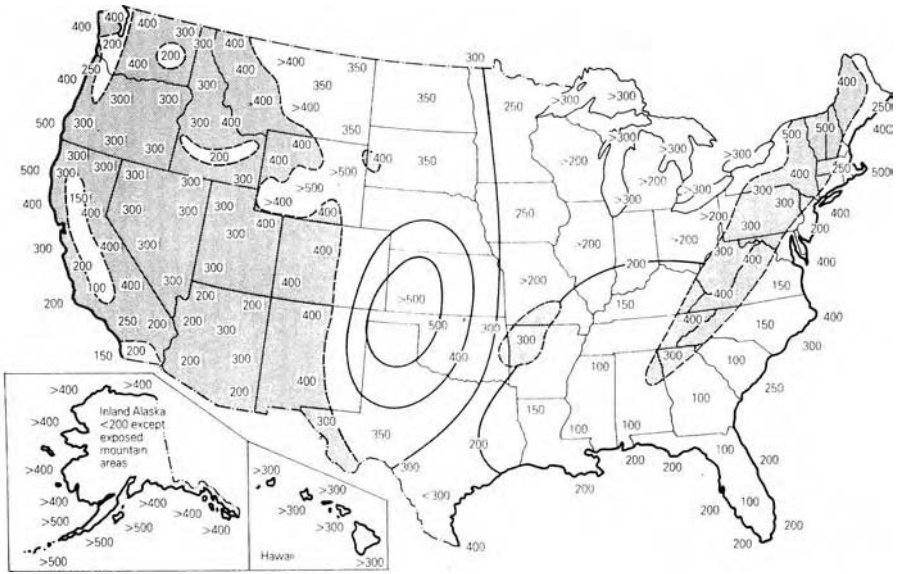
FIGURE 3.17 Annual average wind power density in W/m^2 in the U.S. at 50-m tower height. (From DOE/NREL.)
