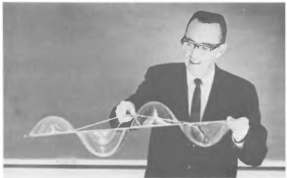
Fig. 6-12 Normal modes of soap film. (Demonstrated by Prof. A. M. Hudson, using a specially strong soap film solution compounded of detergent, glycerin, and a little sugar.)
