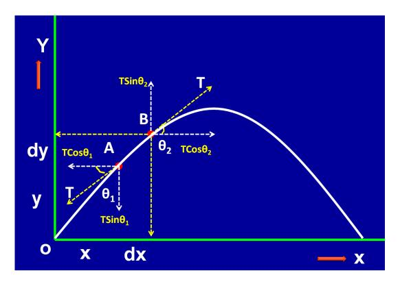
From the figure; at A the tension in the horizontal direction is  $T\cos\theta_1$  and in the vertical direction is  $T\sin\theta_1$ . Similarly at B tension in the horizontal direction is  $T\cos\theta_2$  and in the vertical direction is  $T\sin\theta_2$ . Hence  $T\cos\theta_1$  and  $T\cos\theta_2$  are nearly equal and balance each other.
