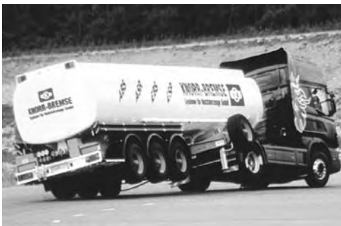
Fig. 9.12. A truck trailer combination on the stability limit, by Knorr Bremse.
