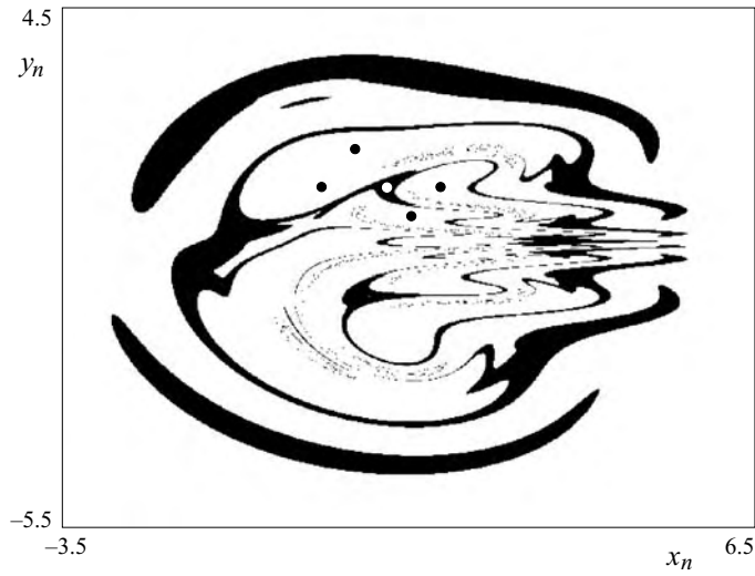
Fig. 9.15. Basins of attraction of the active (white) and inactive summer (black) in the plane of initial conditions with z = 0 ( F = 6 ). The active summer attractor is represented on this plane by four points marked by black dots (cf. Fig. 9.14(b), y vs. t ). The inactive summer attractor appears as a white dot. Note that the inactive basin is much smaller than the active one and that it does not extend towards large values of the variables.
