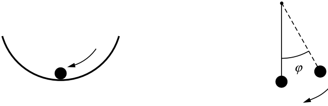
Fig. 3.6. Stable states: a ball placed at the bottom of a concave surface and a pendulum. Rest is only possible at a single point, but, if the system is displaced, it starts moving towards the equilibrium point.
