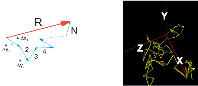
Figure 5.3 Left: A schematic of the N steps in a random walk simulation that end up a distance R from the origin. Notice how the \Delta x 's for each step add algebraically. Right: A simulated walk in 3-D from Walk3D.py .
