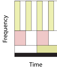
Figure 11.7 A graphical representation of the relation between time and frequency resolutions (the uncertainty relation). Each box represents an equal portion of the time–frequency plane but with different proportions of time and frequency.
