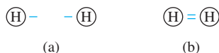
Figure 1.16 | Representation of (a) hydrogen valence electrons and (b) covalent bonding in a hydrogen molecule.
