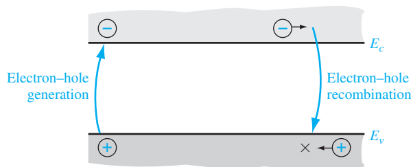
Figure 6.1 | Electron-hole generation and recombination.
