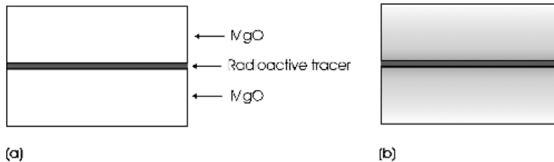
Figure 7.2 A diffusion couple formed by two crystals of \text{MgO} separated by radioactive material: (a) initially and (b) after heating
