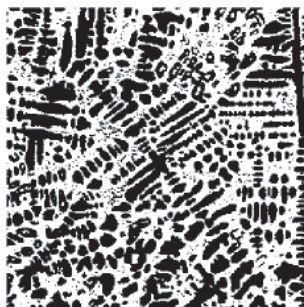
Figure 4.1.9 Micrograph of a multi-phased alloy.
