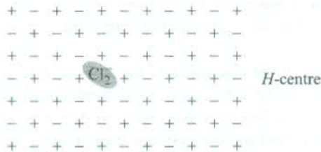
FIG. 12.10 The H -centre—an interstitial chlorine ion bound by a hole to a symmetrically situated lattice chlorine ion. The resulting singly-ionized chlorine molecule occupies a single chlorine ion site.
