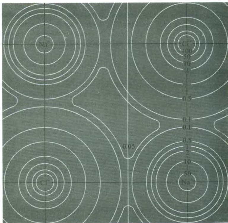
FIG. 2.2 Electron density distribution in the basal plane of NaCl. The numbers of contours express the relative electron density. [From Kittle, C., An Introduction to Solid State Physics , 6th ed., p. 65, John Wiley (1986).]
