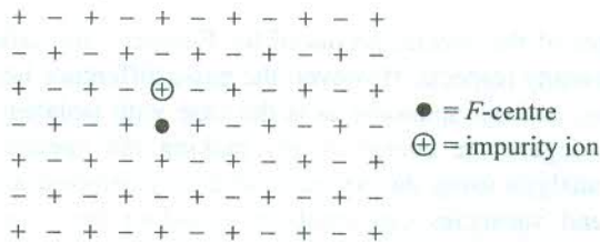
FIG. 12.8 The F_A -centre—an impurity ion replacing one of the six nearest-neighbour positive ions that surround an F -centre.
