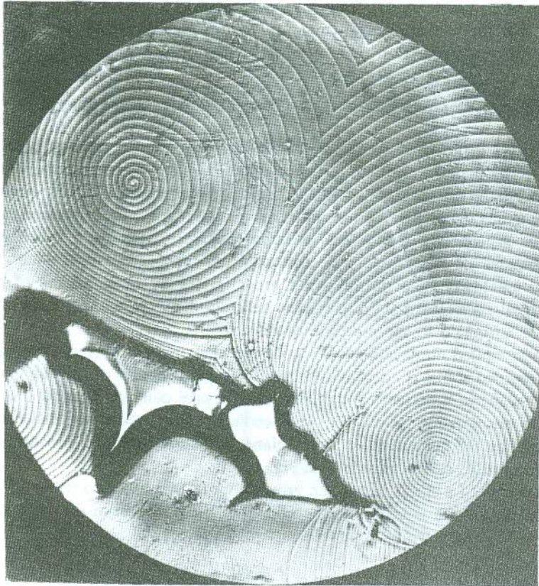
FIG. 12.27 Phase contrast micrograph of spiral growth pattern in SiC crystal of 126 R unit cell modification (rhombohedral). Step height, h = 109 \pm 5 \text{ \AA} (Mag. \times 90 ). (Courtesy A.R. Verma)
