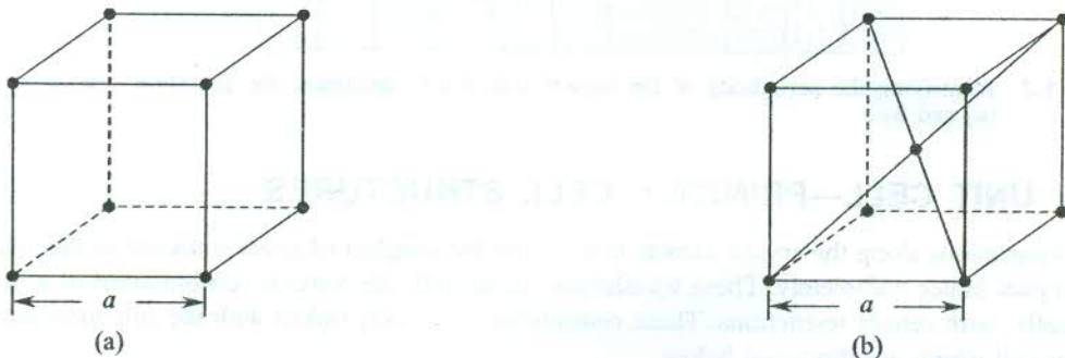
FIG. 1.4 (a) A primitive cell. There is one lattice point in the cell. A point at the corner of the cube contributes the fraction (1/8) . (b) A non-primitive cell with two lattice points per cell.
