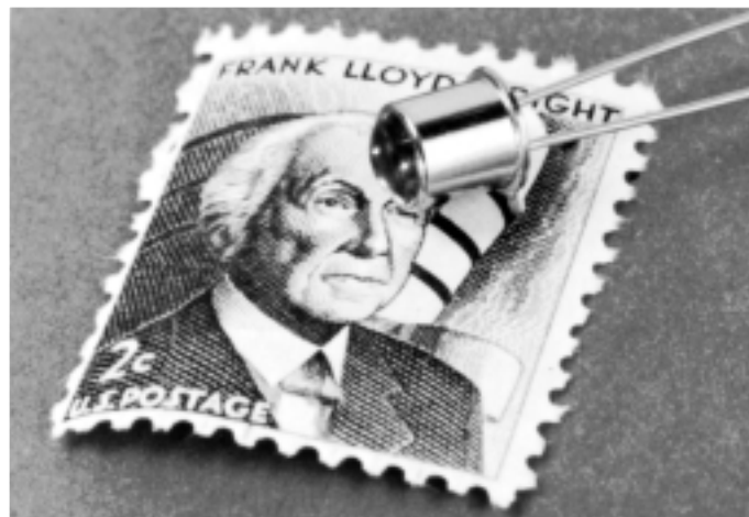
Figure 20.34 RCA IR-emitting diode: (a) construction; (b) photo; (c) symbol. (Courtesy RCA Solid State Division.)
