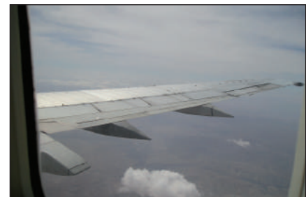
(b) Flaps retracted (cruising)
