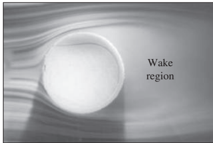
FIGURE 11-15 Flow separation and the wake region for flow over a tennis ball. NASA and the Cislunar Aerospace, Inc.
